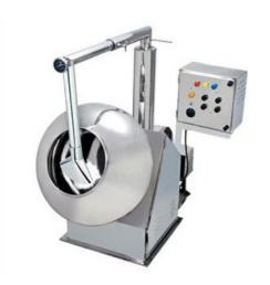
Our range of tablet coating pans is extensively used for sugar and film coating of tablets, pallets and granules. The unit comprises of ellipsoidal shaped pan fabricated using stainless steel sheet and mounted on the gearbox shaft, which is driven by an electric motor.
