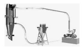
Vacuum transfer systems are ideal for long distance conveying and where product degranulation is a concern.
